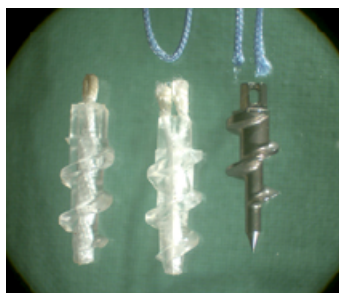
Figure 2: Biocorkscrew and Corkscrew anchors demonstrating the eyelets and failure mode.
