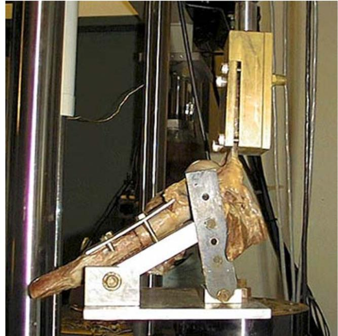
**Fig. 1** Test set up demonstrating custom-made jig to alter the abduction angle
