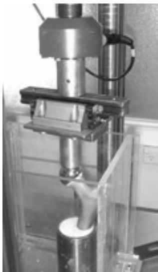
Figure 1 A resurfaced femur is tested using a MTS 858 testing system.
